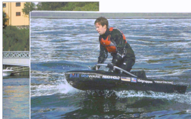
Evolo is a hydro toy powered by a 4 kW electric motor and 16 3V battery cells. Dimensions 2.31 x 0.7 meters. At the bottom of the 80 cm long buttress are the delta-shaped carrier planes.
